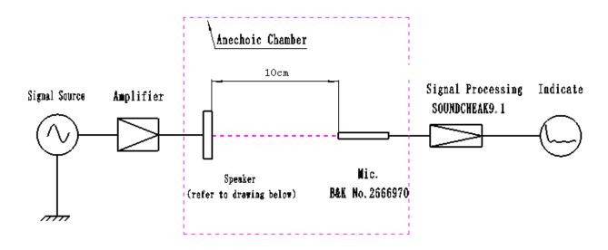
The speaker, being tested in an anechoic chamber, is installed in a baffle of 135cmx165cm. Conditions of testing:
